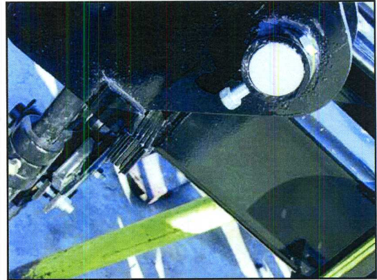
REMOVABLE SPACER'S FOR WING TILT
