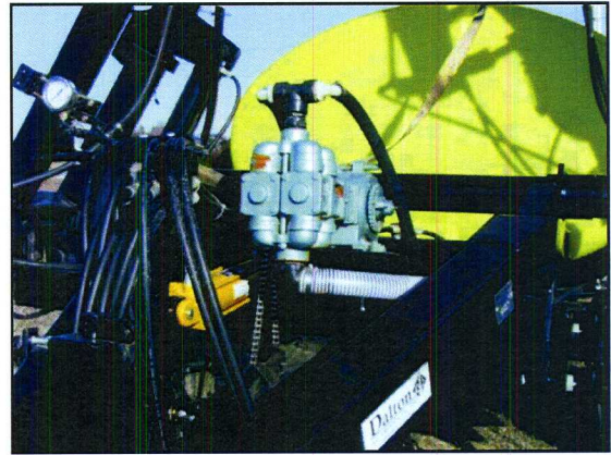
TEE ON DISCHARGE SIDE OF PUMP WITH 2-FEEDER LINES TO BOOM HOSE, 2" ST EL HOSEBARB IN SUCTION SIDE OF PUMP
