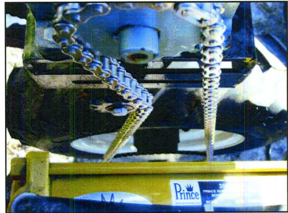
TIGHTNER ON SLACK SIDE OF PUMP DRIVE CHAIN
