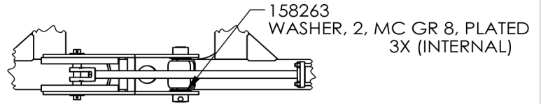
TOP VIEW, INBOARD HINGE
